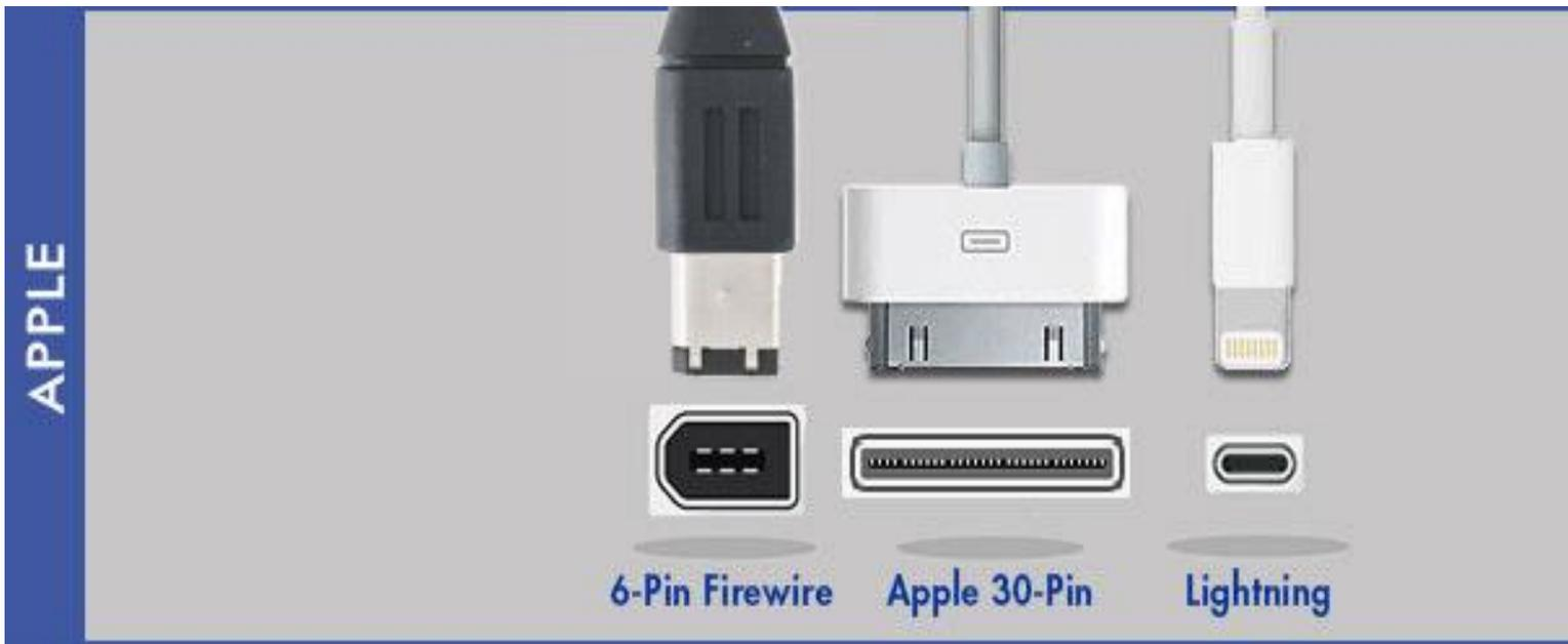
**6-Pin FireWire Connector:** This was the connector of the original iPod, and was used until the third-generation iPod introduced a new dock connector. Although the original iPod had dock-to-FireWire capabilities, Apple eventually phased out all FireWire in favor of a USB version.
